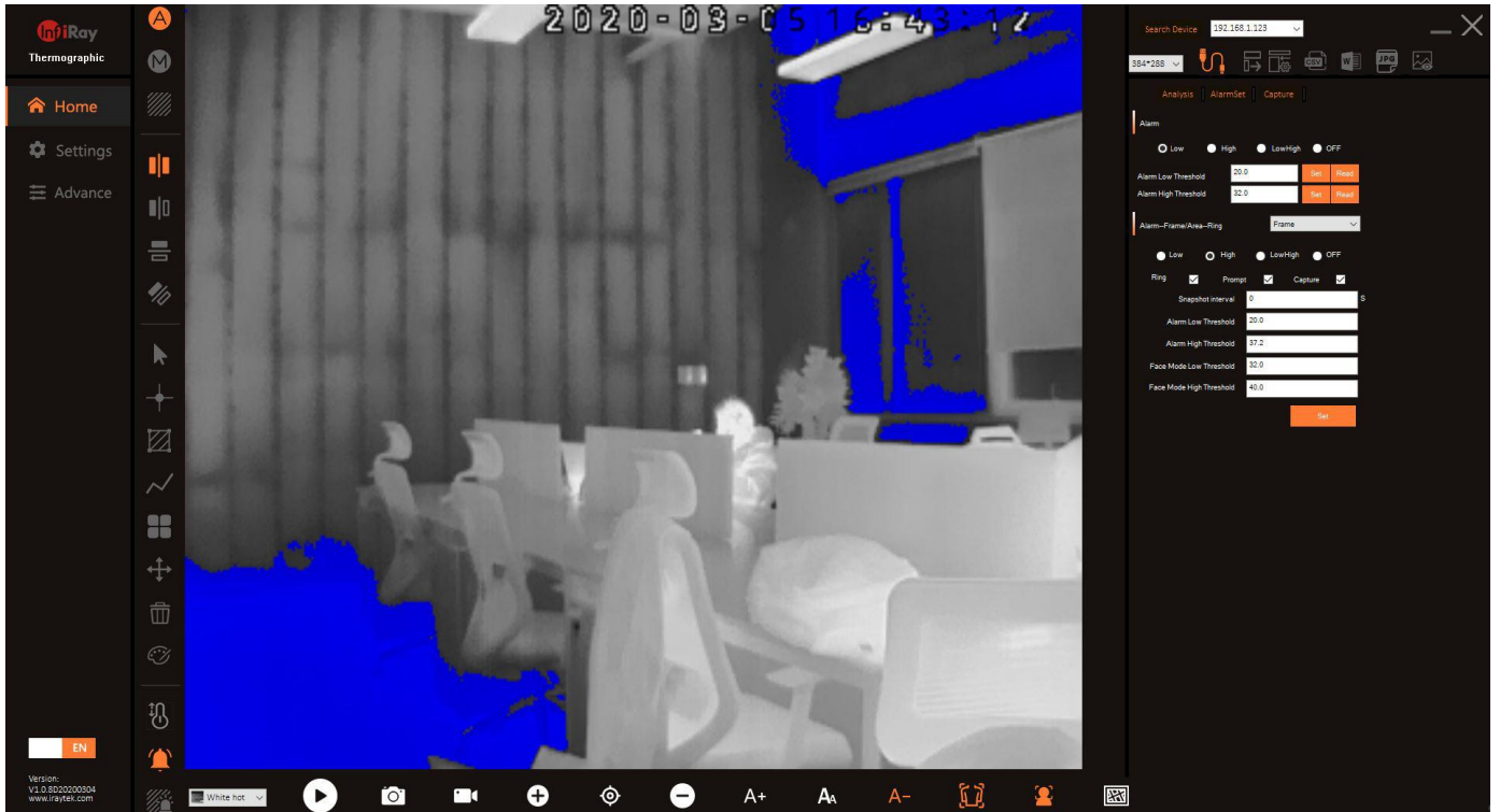
Figure 2.9 Setting--Temperature measurement setting --- Low temperature alarm
